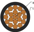
Bare copper conductor LSOH cross-link polyolefin insulation
